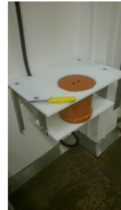
Ear tag reader manufactured by Shearwell and used at Linden Foods
